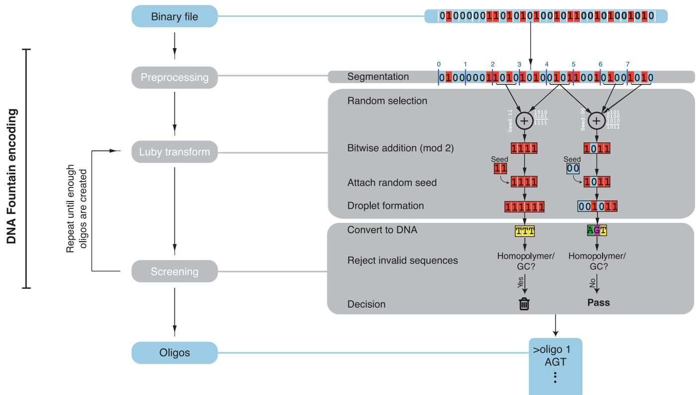
**Fig. 1. DNA Fountain encoding.** (Left) Three main algorithmic steps. (Right) Example with a small file of 32 bits. For simplicity, we partitioned the file into eight segments of 4 bits each. The seeds are represented as 2-bit numbers and are presented for display purposes only. See (12) for the full details of each algorithmic step.
