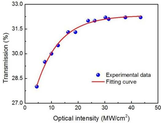
Fig. 2. The nonlinear transmission characteristic of the TISA.
