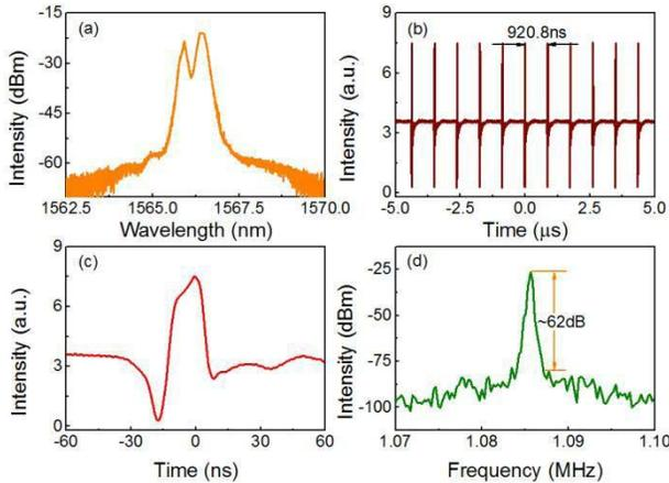
Fig. 4. Typical optical characteristics of the bright-dark soliton pair at the pump power of 97.3 mW. (a) the output optical spectrum; (b) the pulse train; (c) the corresponding single pulse profile of the bright-dark soliton pair and (d) the corresponding RF spectrum.
