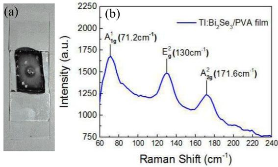
Fig. 1. (a) The photograph and (b) the Raman spectrum of the TI:  $\text{Bi}_2\text{Se}_3/\text{PVA}$  film.
