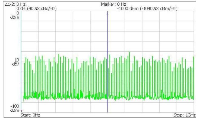
Fig. 5. The RF spectrum of the bright-dark soliton pair measured in wider frequency range (1GHz).
