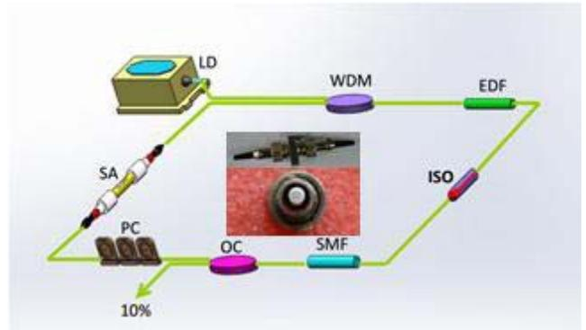
Fig. 3. The experimental setup of our proposed fiber laser. Inset: top, the photograph of the mode-locker; bottom, the photograph of the pigtail with the TI:  $\text{Bi}_2\text{Se}_3/\text{PVA}$  film (gray color).
