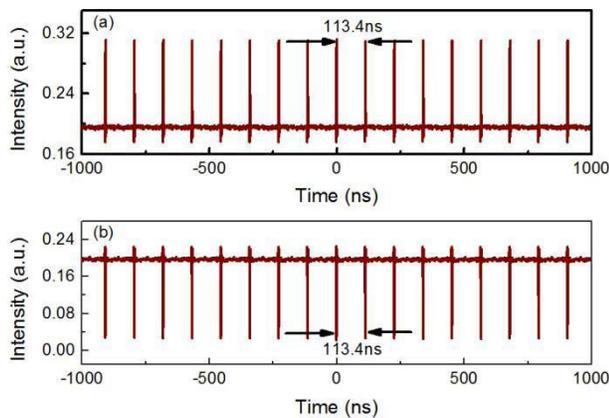
Fig. 7. Separated measurement of the pulse train of the bright-dark soliton pair under the external cavity rotatable polarizer. (a) the bright soliton; (b) the dark soliton when  $L_{SMF} = 18.3$  m,  $\beta_{2,cavity} = \sim -0.32$  ps<sup>2</sup>.
