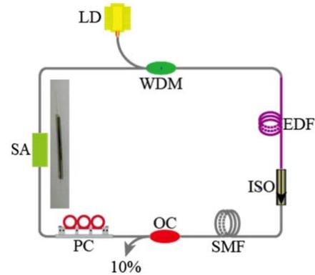
Fig. 3. Experimental setup. Inset: the photograph of the WS<sub>2</sub>-based fiber taper.
