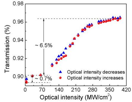
Fig. 2. The nonlinear saturable absorption curve of the WS<sub>2</sub>-based fiber taper: the blue color and red color represents optical intensity of pump laser decreasing and increasing, respectively.
