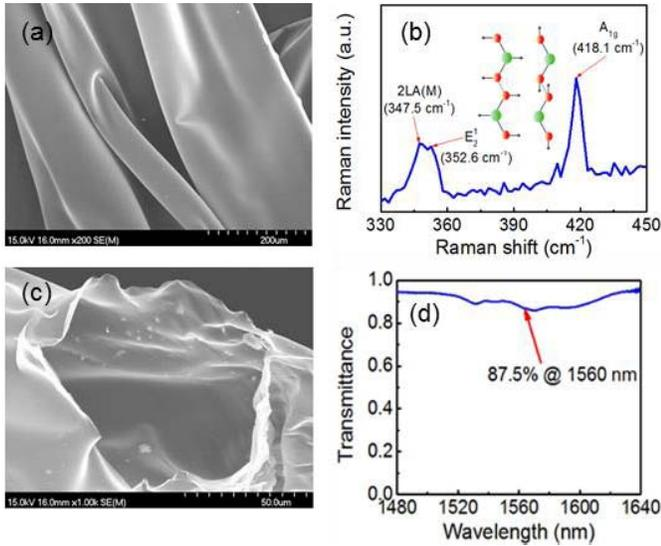
Fig. 1. Typical characteristics of the 2D WS<sub>2</sub> film: (a) and (c) show the SEM image of sample with the resolution of 200  $\mu\text{m}$  and 50  $\mu\text{m}$ , respectively; (b) the Raman spectrum of WS<sub>2</sub> film; (d) the linear absorption spectrum of WS<sub>2</sub> film.
