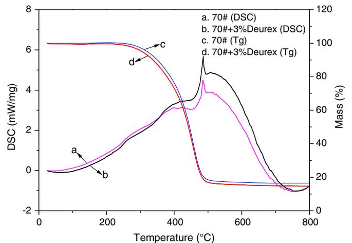
**Fig. 13.**  $T_g$ -DSC curves for binders with and without Deurex
