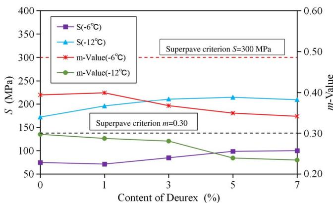
Fig. 8. Creep stiffness ( $S$ ) value and  $m$  value variations with changes in additive content at  $-6$  and  $-12$ °C
