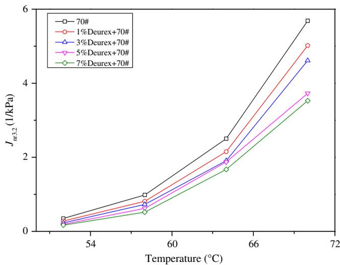
**Fig. 12.** Variations in nonrecoverable creep compliance ( $J_{nr3.2}$ ) with changes in additive content at four test temperatures
