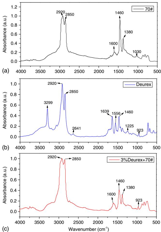
**Fig. 14.** FTIR analysis: (a) base asphalt; (b) Deurex; (c) 3% Deurex-modified asphalt
