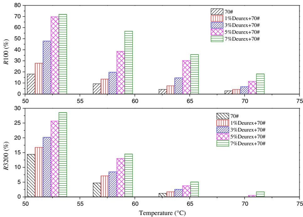
**Fig. 11.** Variations in  $R_{100}$  and  $R_{3200}$  with changes in additive content at four test temperatures
