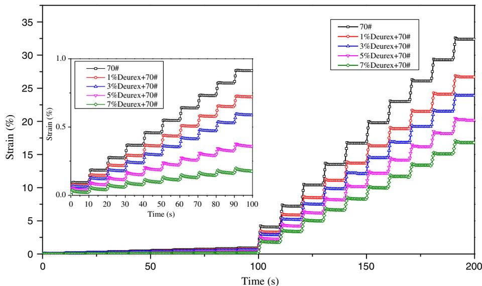
Fig. 10. MSCR test at 58°C
