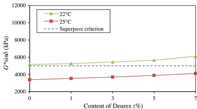
Fig. 7.  $G^* \sin \delta$  values for RTFO + PAV aged WMA binders
