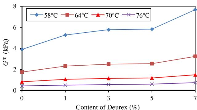
Fig. 4. Complex shear modulus  $G^*$
