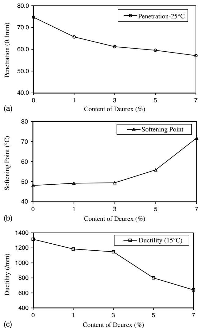
**Fig. 2.** Conventional properties of Deurex-modified asphalt binder: (a) penetration at 25°C; (b) softening point; (c) ductility at 15°C
