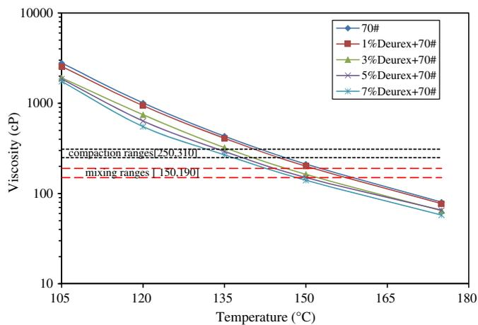
Fig. 3. Rotational viscosity test
